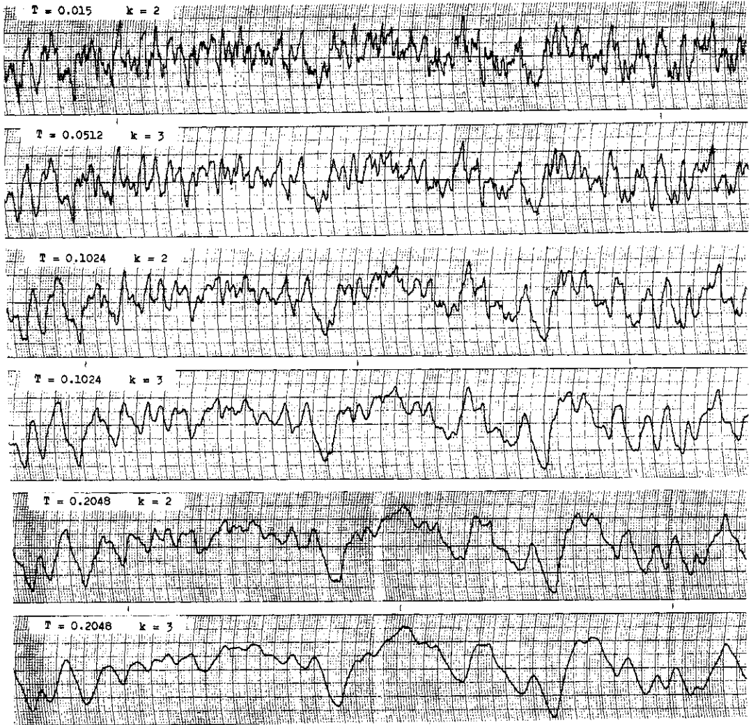
Fig. 3. Noise N_T^k made from white noise (series of random numbers) by k operations of first-order lag system having time constant T .
