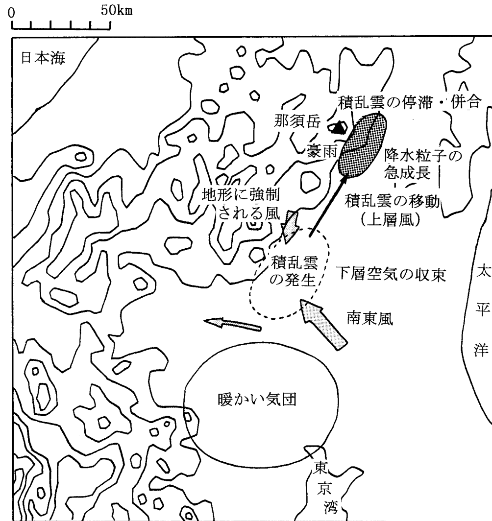
図18 降雨が集中する過程の模式図 Fig.18 A schematic illustration of the process of the heavy rainfall.
