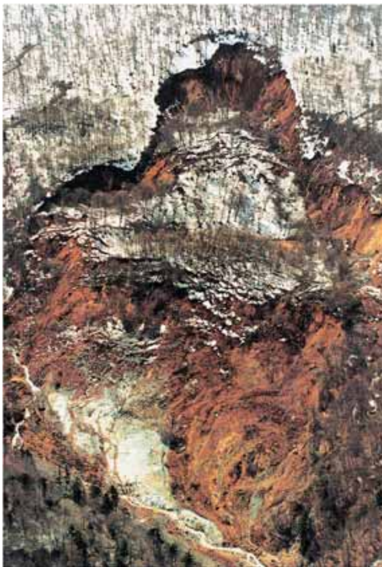
Fig. 3.14 An overview of Sumikawa Onsen landslide and debris avalanche. The landslide occurred at a part of landslide topographic area (Half of the body remains at the area and the rest moved away as a debris avalanche to the 2km downstream).
