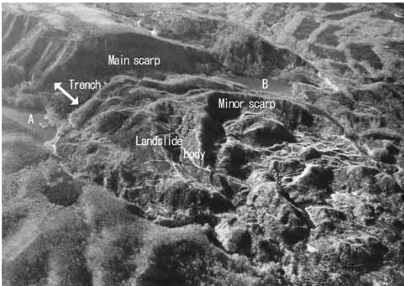
Fig. 5.5 An overview of typical "large scale landslide topography". Shironuma landslide area distribute at the foot slope of the Funagata volcano, Miyagi Prefecture northeast Japan.
